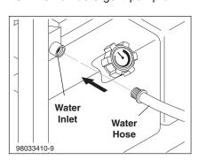
STEP 7: Connect the other end of the water hose to pump water inlet. Inspect inlets. *CAUTION: Do not* run the pump without water or pump damage will result.
