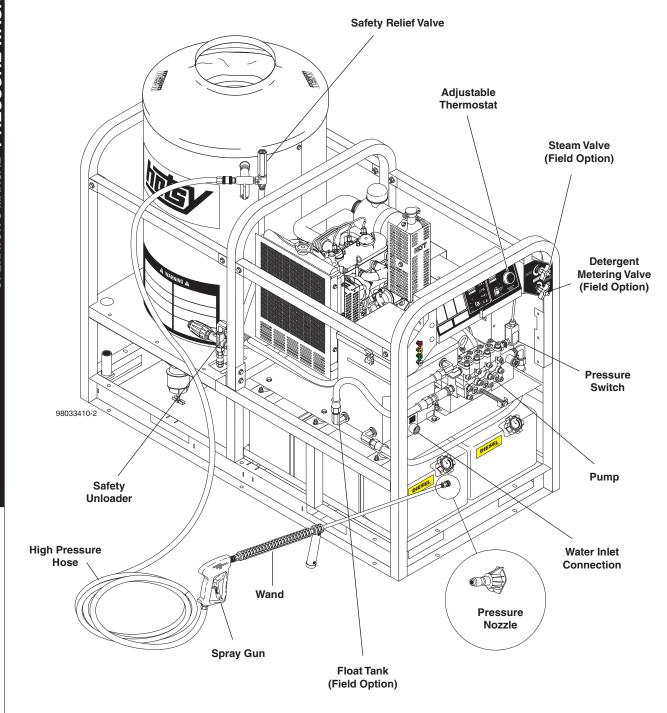
**Pump** — Develops high pressure by pumping water volume through nozzle.
