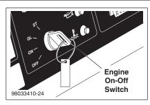
**STEP 2:** Turn key to stop position. Engine shuts down by way of solenoid.
