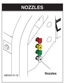
The quick connect nozzles provide a wide array of spray widths from 0° to 40° and are easily accessible when placed in the convenient rubber nozzle holder, which is provided on the front of the machine.
