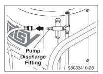
**STEP 6:** Disconnect the high pressure hose from pump discharge fitting.
