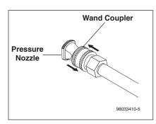
**STEP 3:** Release the coupler collar and push the nozzle in until the collar clicks. Pull the nozzle to make sure it is seated properly.
