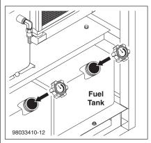
**STEP 2:** Fill engine/burner fuel tanks with fuel.
