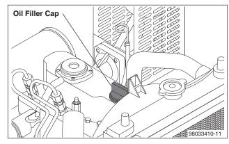
**STEP 1:** Check engine oil level. Oil level should be between the lines on the dipstick. (Refer to the engine's operating manual included with machine.) We recommend that the oil be changed after the first 5 hours of use, then once every 50 hours. **NOTE:** Improper oil levels will cause low oil sensor to shut off engine. **IMPORTANT! Do not run engine with high or low oil levels as this will cause engine damage.**
