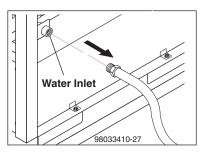
**STEP 5:** Disconnect the water supply from the water inlet on the machine.
