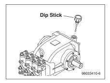
**STEP 4:** Remove shipping cap and install oil dipstick. Check pump oil level by using dipstick or observe oil level in oil window (if equipped). Use 10W-40 non detergent pump oil.
