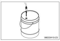
**STEP 1:** Remove detergent suction tube from container and insert into one gallon of fresh water. Open detergent mixing valve. Pull trigger on spray gun and siphon water for one minute.
