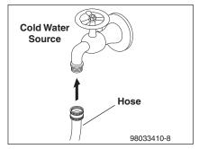
**STEP 6:** Connect one end of hose to the cold water source.
