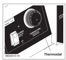
Step 2: Turn the thermostat knob to the 270° mark, (The thermostat is a high limit device and does not regulate temperature).
