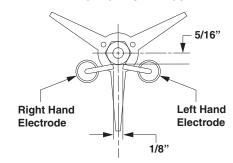
Periodically Check Wiring Connections. If Necessary to adjust electrodes, use diagram.
