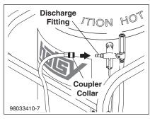
**STEP 5:** Connect the high pressure hose to the pump discharge fitting. Push coupler collar forward until secure.
