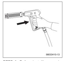
**STEP 3:** Before installing nozzle, trigger the spray gun to eliminate trapped air then wait for a steady flow of water to emerge from the wand coupler when engine starts. Run machine allowing water to flush through the system until clear.
