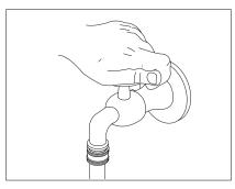
**STEP 2:** Before installing nozzle, turn on water supply and run machine allowing water to flush through the system until clear.
