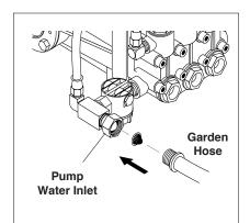
STEP 7: Check inlet filters, remove debris, then connect garden hose to pump water inlet. CAUTION: Do not run the pump without water or pump damage will result.
