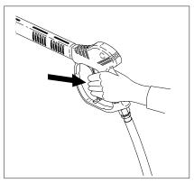
**STEP 4:** Trigger the spray gun to eliminate trapped air then wait for a steady flow of water to emerge from the spray nozzle.
