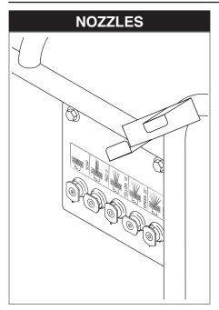
The five color-coded quick connect nozzles provide a wide array of spray widths from 0° to 40° and are easily accessible when placed in the convenient rubber nozzle holder, which is provided on the front of the machine.
