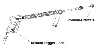
*IMPORTANT: The trigger gun provided with this pressure washer is equipped with a manual trigger lock to prevent accidental operation of the trigger gun. The trigger lock should be used whenever the trigger gun is not in use.*
