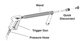
3. Assemble wand components as shown.
